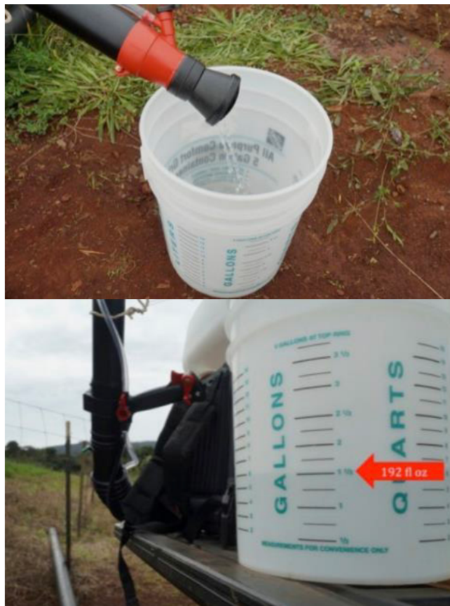
Figure 6: Measuring the amount of water remaining in the tank or hopper will help you calculate the amount of water used to spray the sample trees as well as to estimate water usage in gallons per acre.
