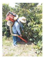
Fig. 1. Vacuum machine prototype to collect coffee berries from the ground.
