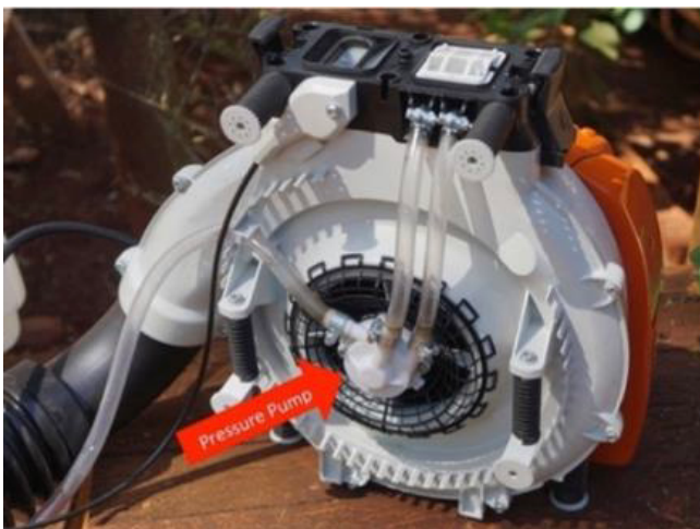
Figure 5: An example of a pressure pump kit installed on a mist blower to maintain consistent output.
