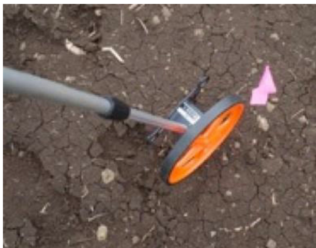
Figure 3: Using a contractor's measuring wheel can help to calculate field area and acreage.
