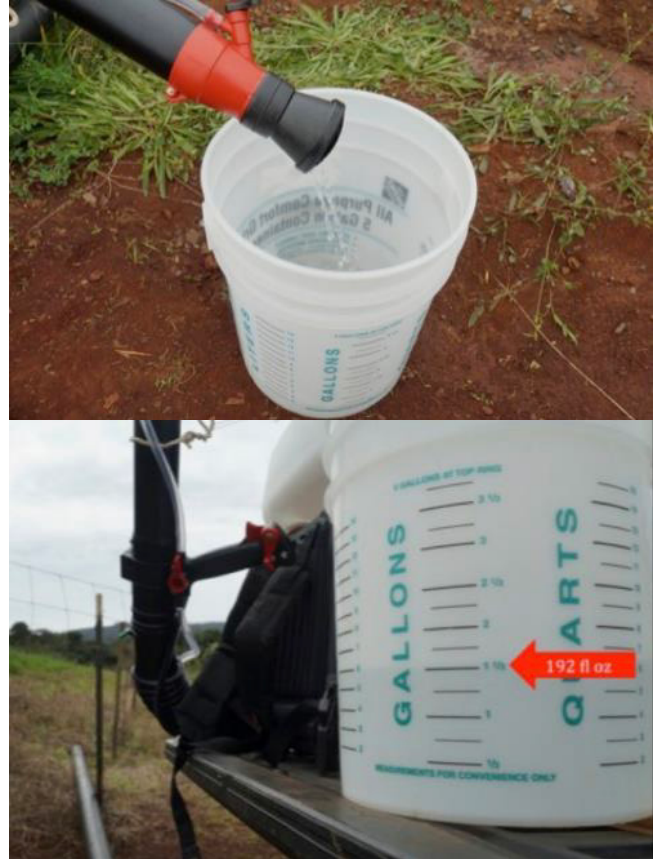
Figure 6: Measuring the amount of water remaining in the tank or hopper will help you calculate the amount of water used to spray the sample trees as well as to estimate water usage in gallons per acre.
