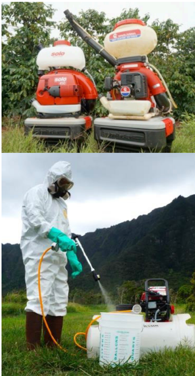
Figure 1: Examples of handheld sprayer systems used on orchard crops. Backpack mist blower (top) and motorized tank sprayer with hose and wand attachment (bottom).
